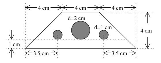
*Clearly* demonstrate the process by which you could locate the centroid of the plate below. You may assume that the material has uniform density. Once you have found the location of the centroid, draw a \* at approximately that location on the drawing. Note that the plate has left-right symmetry and that the bottoms of the three circles are aligned.
