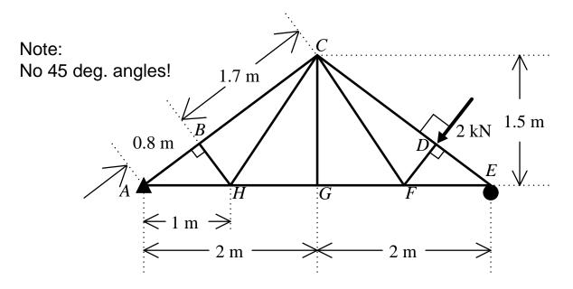
and assuming that there is a 2 kN force directed perpendicular to CDE at node D,
