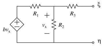
and assuming that the values for the passive elements  $(R_1, R_2, R_3)$  and the value for the constant b are known, find expressions for  $v_{\rm Th}$ ,  $i_{\rm N}$ , and  $R_{\rm Th}$ , then draw the Thévenin and Norton circuit with respect to terminals  $\xi$  and  $\eta$  in terms of the known values. Be sure to show your process clearly and indicate where  $\xi$  and  $\eta$  are in your equivalent circuit drawings.
