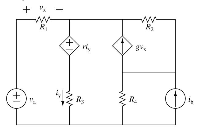
and assuming that constants r and g, the values for the passive elements ( $R_1$  through  $R_4$ ), and the values for the independent sources ( $v_a$  and  $i_b$ ) are known,
