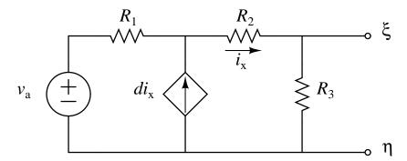
and assuming that the values for the passive elements ( $R_1$  and  $R_2$ ), the value for the source ( $v_a$ ), and the value for the constant d are known, draw the Norton equivalent circuit with respect to terminals  $\xi$  and  $\eta$  in terms of the known values. Be sure to show your process clearly and indicate where  $\xi$  and  $\eta$  are in your equivalent circuit drawings.
