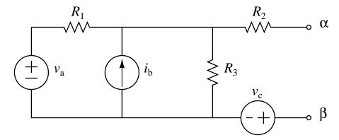
and assuming that the values for the passive elements ( $R_1$  through  $R_3$ ) and the values for the independent sources ( $v_a$ ,  $i_b$ ,  $v_c$ ) are known, draw both the Thévenin and Norton equivalent circuits with respect to terminals  $\alpha$  and  $\beta$  in terms of the known values. Be sure to show your process clearly and indicate where  $\alpha$  and  $\beta$  are in your equivalent circuit drawings.
