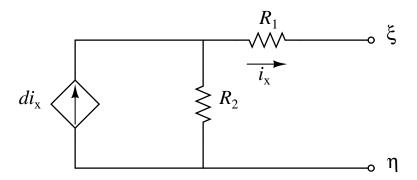
and assuming that the values for the passive elements  $(R_1 \text{ and } R_2)$  and the value for the constant d are known, draw the Norton equivalent circuit with respect to terminals  $\xi$  and  $\eta$  in terms of the known values. Be sure to show your process clearly and indicate where  $\xi$  and  $\eta$  are in your equivalent circuit drawings.
