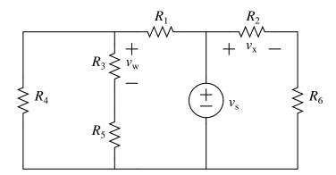
clearly show voltage division to obtain expressions for  $v_{\rm w}$  and  $v_{\rm x}$  in terms of the resistors and  $v_{\rm s}$ .
