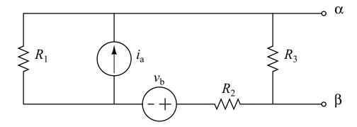
and assuming that the values for the passive elements ( $R_1$  through  $R_3$ ) and the values for the independent sources ( $i_a$  and  $v_b$ ) are known, draw the Thévenin equivalent circuit with respect to terminals  $\alpha$  and  $\beta$  in terms of the known values. Be sure to show your process clearly and indicate where  $\alpha$  and  $\beta$  are in your equivalent circuit drawings.
