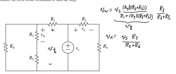
clearly show voltage division to obtain expressions for  $v_{\rm w}$  and  $v_{\rm x}$  in terms of the resistors and  $v_{\rm s}$ .
