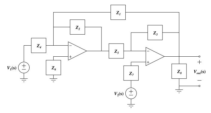
clearly label the circuit and determine a set of equations that could be solved to find an expression for the Laplace transform of the output voltage  $(\mathbb{V}_{\text{out}}(s))$  as a function of the Laplace transform of the input voltages  $(\mathbb{V}_1(s))$  and  $\mathbb{V}_2(s)$  and the impedances  $\mathbb{Z}_k$ . List the total set of unknowns your equations would solve. You are not required to actually solve.
