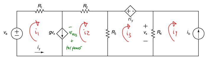
and assuming that constants g and r, the values for the passive elements  $(R_1 \text{ through } R_4)$ , and the values for the independent sources  $(v_a \text{ and } i_b)$  are known,
