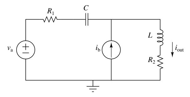
and assuming the circuit has been in place for a very long time, find an expression for the steady-state value of the output current,  $i_{\text{out}}(t)$ , if the sources and passive elements have the following values:
