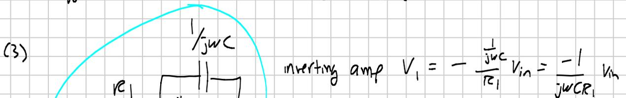
inverting amp  $V_1 = -\frac{1/j\omega C}{R_1} V_{in} = \frac{-1}{j\omega C R_1} V_{in}$
