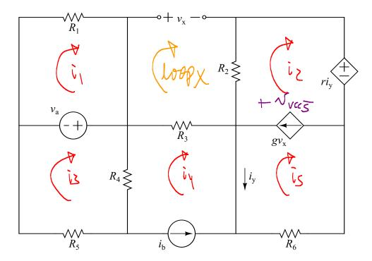
and assuming that constants g and r, the values for the passive elements ( $R_1$  through  $R_6$ ), and the values for the independent sources ( $v_a$  and  $i_b$ ) are known,
