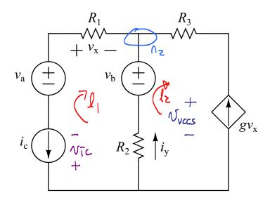
and assuming that constant g, the values for the passive elements ( $R_1$  through  $R_3$ ), and the values for the independent sources ( $v_a$ ,  $v_b$ , and  $i_c$ ) are known, determine expressions for the following items in terms of known values. Note - if you solve for an unknown in terms of known quantities and clearly indicate that expression, you may use that unknown in later calculations without substitution. Put your expressions next to the appropriate bullet below:
