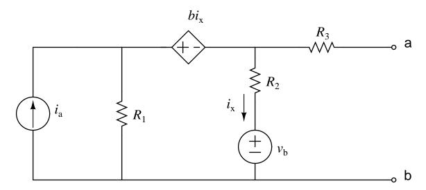
and assuming that gain b, the values for the passive elements  $(R_1, R_2, R_3)$ , and the values for the independent sources  $(i_a, v_b)$  are known, draw both the Thévenin and Norton equivalent circuits with respect to terminals a and b in terms of the known values.
