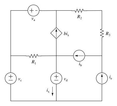
and assuming that gain b, the values for the passive elements  $(R_1, R_2, R_3)$ , and the values for the independent sources  $(v_a, i_b, v_c, v_d, i_e)$  are known, determine expressions for the following values in terms of known values. Note - if you solve for an unknown in terms of known quantities and clearly indicate that expression, you may use it in later calculations without substitution. Put your expressions next to the appropriate bullet below:
