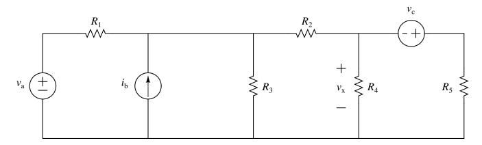
and assuming that the values for the passive elements  $(R_1, R_2, R_3, R_4, R_5)$ , and the values for the independent sources  $(v_a, i_b, v_c)$  are known, *clearly* demonstrate the use of superposition and find an expression for the unknown voltage  $v_x$  in terms of the passive element values and the sources.
