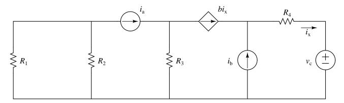
and assuming that gain b, the values for the passive elements, and the values for sources  $i_a$ ,  $i_b$ , and  $v_c$  are known, determine expressions for the power absorbed by each of the four sources in terms of known values. Note - if you solve for an unknown in terms of known quantities and clearly indicate that expression, you may use it in later calculations without substitution. Put your expressions next to the appropriate bullet below:
