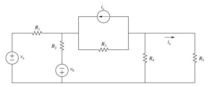
and assuming that the values for the passive elements as well as sources  $v_a$ ,  $v_b$ , and  $i_c$  are known, clearly demonstrate the use of superposition and find an expression for the unknown current  $i_x$  in terms of the passive element values and the sources.
