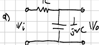
$$\frac{V_o}{V_i} = \frac{\frac{1}{jwC}}{R + \frac{1}{jwC}} = \frac{1}{1 + jwCR} = \frac{1/RC}{jw + 1/RC}$$
