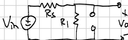
is just a voltage divider,  $\frac{R_1}{R_1+R_s}$
