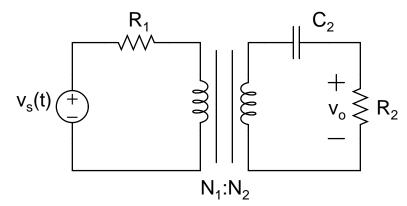
Given the circuit above and known values  $v_s(t)$ ,  $C_2$ ,  $R_1$ ,  $R_2$ ,  $N_1$ , and  $N_2$ , find the network function:
