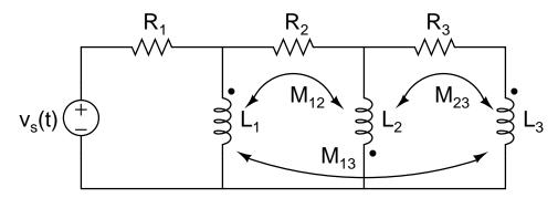
Given the circuit above and known values  $v_s(t)$ ,  $L_1$ ,  $L_2$ ,  $L_3$ ,  $M_{12}$ ,  $M_{13}$ ,  $M_{23}$ ,  $R_1$ ,  $R_2$ ,  $R_3$ , write the three mesh current equations in the frequency domain or in the time domain.
