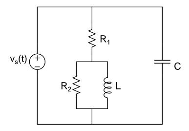
Assume you add a 5  $\mu F$  capacitor in parallel with the voltage source as shown above.
