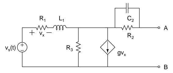
(2) Given the circuit above and the known values  $v_{\rm s}(t)$ ,  $C_2$ ,  $L_1$ ,  $R_1$ ,  $R_2$ ,  $R_3$ , and g, find  $\mathbb{V}_{\rm oc}$ ,  $\mathbb{I}_{\rm sc}$ , and  $\mathbb{Z}_{\rm th}$  as seen across terminals A-B.
