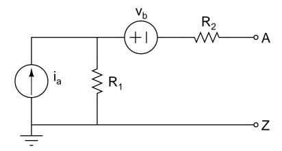
and known values  $i_a$ ,  $v_b$ ,  $R_1$ , and  $R_2$ , determine and draw both the Thévenin and Norton equivalent circuits as seen at terminals AZ.
