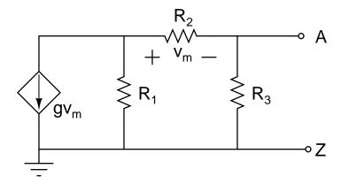
and known values g,  $R_1$ ,  $R_2$ , and  $R_3$ , determine and draw the Thévenin equivalent circuit as seen at terminals AZ.
