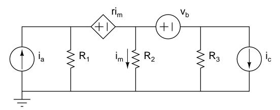
and known values  $i_a$ ,  $v_b$ ,  $i_c$ , r,  $R_1$ ,  $R_2$ , and  $R_3$ , find  $i_m$  using superposition. You *must* redraw the circuit each time to get full credit for this problem.
