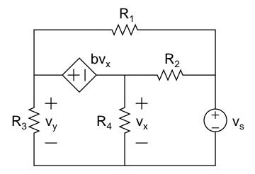
and known values  $v_s$ , b,  $R_1$ ,  $R_2$ ,  $R_3$ , and  $R_4$ , find  $v_y$  in terms of the known values using the Node Voltage Method.
