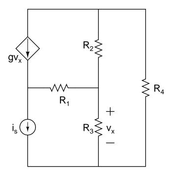
and known values  $i_s$ , g,  $R_1$ ,  $R_2$ ,  $R_3$ , and  $R_4$ , find  $p_{{\rm abs},R_4}$  in terms of the known values using the Mesh Current Method. Hint: use the two simple-source equations first to get a single equation for the unknown current in the tallest mesh.
