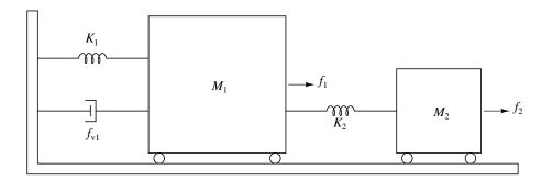
and assuming  $f_1$ ,  $f_2$ , and the spring, mass, and damper values are known, clearly define your state variables and write the state space equations for the circuit using those variables. The desired output for this system will be the position of mass  $M_2$ .
