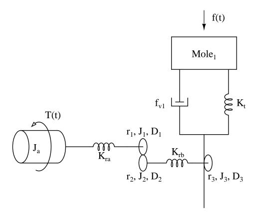
is one model of the famous "Whack-A-Mole" game. Torque T(t) is used to provide the effort needed to lift the mole up through a hole in the playing board. The rotational and translational shafts have stiffnesses represented by the various springs and the gears are all supported by housings which, among other things, provide damping. Force F represents the force applied by the mallet when a player attempts to whack said mole. Damper  $f_{v1}$  is in place to cushion the blow.
