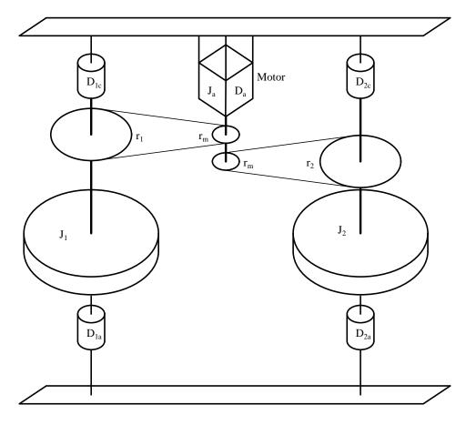
where the dampers  $D_{1c}$  and  $D_{2c}$  represent the viscous damping between the unmoving ceiling and the rotating fan shafts, dampers  $D_{1a}$  and  $D_{2a}$  represent the viscous damping resulting from air flow, and the inertias  $J_1$  and  $J_2$  represent the rotational inertias of both the fan shafts and the fan blades.
