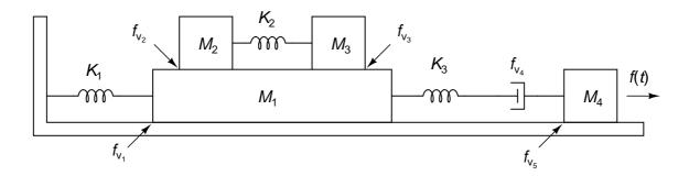
set up, but do not solve, a system of equations that could be used to find a transfer function between the position of anything in the system and the force applied to  $M_4$ . Your answer should be presented in matrix form, and you must clearly indicate what your variables mean.
