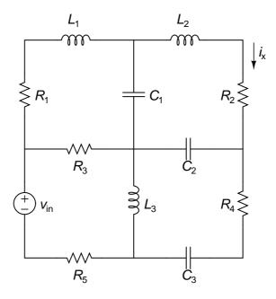
set up, but do not solve, a system of equations that could be used to find a transfer function between the output current and the input voltage. Your answer should be presented in matrix form, and you must clearly indicate what your variables mean.
