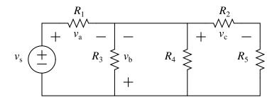
clearly show voltage division to obtain expressions for  $v_{\rm a}$ ,  $v_{\rm b}$ , and  $v_{\rm c}$  in terms of the resistors and  $v_{\rm s}$ .
