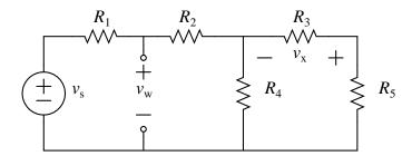
clearly show voltage division to obtain expressions for  $v_{\rm w}$  and  $v_{\rm x}$  in terms of the resistors and  $v_{\rm s}$ .
