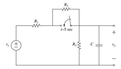
with a switch that is initially open for a very long time before t=5 sec and then closes at t=5 sec and remains closed from that point forward. Assuming that the voltage  $v_{\rm s}(t)$  is a constant 24 V and the values of the reactive elements are
