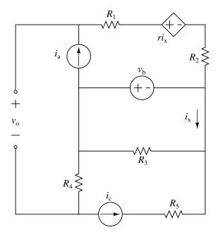
and assuming that constant r, the values for the passive elements ( $R_1$  through  $R_5$ ), and the values for the independent sources ( $i_a$ ,  $v_b$ , and  $i_c$ ) are known, determine expressions for the following values in terms of known values. Note - if you solve for an unknown in terms of known quantities and clearly indicate that expression, you may use it in later calculations without substitution. Put your expressions next to the appropriate bullet below:
