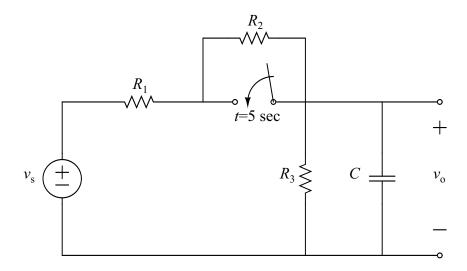
with a switch that is initially open for a very long time before t=5 sec and then closes at t=5 sec and remains closed from that point forward. Assuming that the voltage  $v_s(t)$  is a constant 24 V and the values of the reactive elements are
