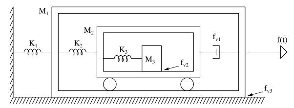
where f(t) is a known force applied to mass  $M_1$  and assuming that the values of the passive elements are known, clearly determine a complete set of equations of motion for the system in the frequency domain. List the set of unknowns you believe your equations use and be sure they are all clearly labeled on the diagram. You do not need to arrange the equations in matrix format nor do you need to solve the equations. You may assume that the wheels are both frictionless and massless.
