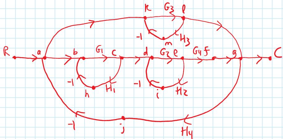
$$T_1: RabcdegC = G_1G_2G_4 \quad L_1: bchb = -G_1H_1$$
