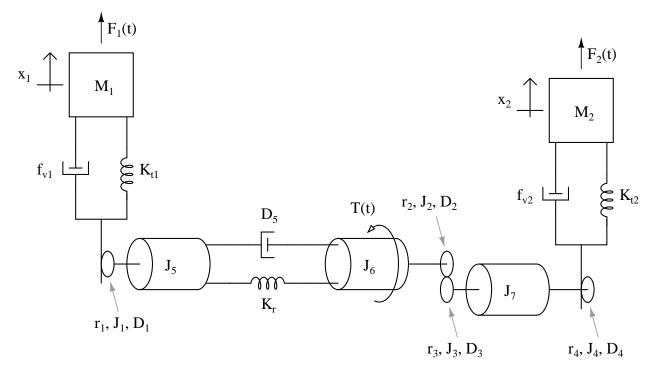
where  $F_1(t)$  is a force applied to mass  $M_1$ ,  $F_2(t)$  is a force applied to mass  $M_2$ , T(t) is a torque applied to rotational inertia  $J_6$ ,  $x_1$  is the position of mass  $M_1$ , and  $x_2$  is the position of mass  $M_2$ ,
