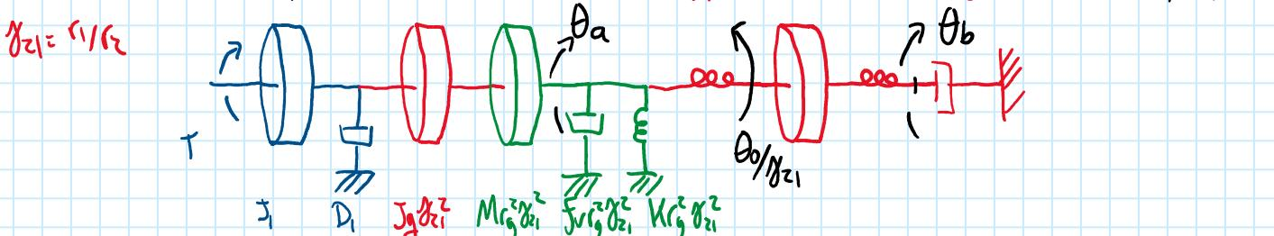
$$a: ((J_1 + \theta_{21}^2 (J_g + M_r_g^2)) s^2 + (D_1 + f_v r_g^2 \gamma_{21}^2) s + (K_r g^2 \gamma_{21}^2 + K_1 \gamma_{21}^2) \dot{\theta}_a - K_1 \gamma_{21}^2 (-\dot{\theta}_o) = T$$
