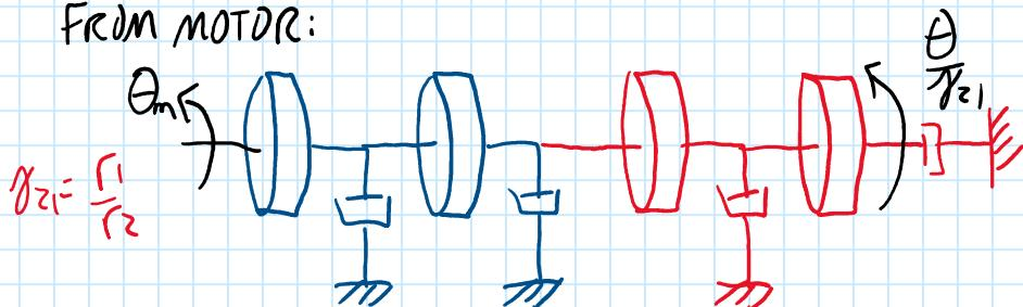
$$J_a \quad D_a \quad J_1 \quad D_1 \quad J_2 \gamma_{zi}^2 \quad D_2 \gamma_{zi}^2 \quad J_c \gamma_{zi}^2 \quad D_3 \gamma_{zi}^2$$
