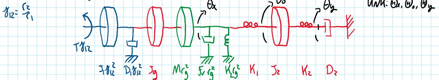
$$x: ((J_1 \gamma_{12}^2 + J_g + M_r_g^2) s^2 + (D_1 \gamma_{12}^2 + f_v r_g^2) s + (K_r g^2 + K_1)) \dot{\theta}_x - K_1 \dot{\theta}_o = -T \gamma_{12}$$
