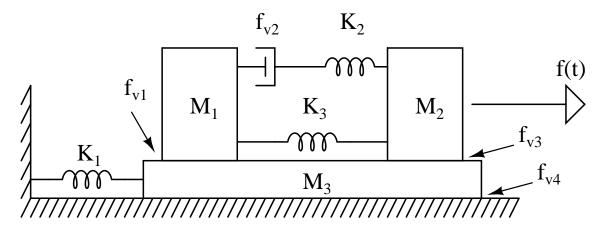
where f(t) is a known force applied to mass  $M_2$  and assuming that the values of the passive elements are known, clearly determine a complete set of equations of motion for the system in the frequency domain. List the set of unknowns you believe your equations use and be sure they are all clearly labeled on the diagram. You do not need to arrange the equations in matrix format nor do you need to solve the equations.
