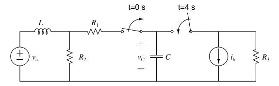
note that the left switch opens at time t=0 s and, four seconds later, the right switch closes.
